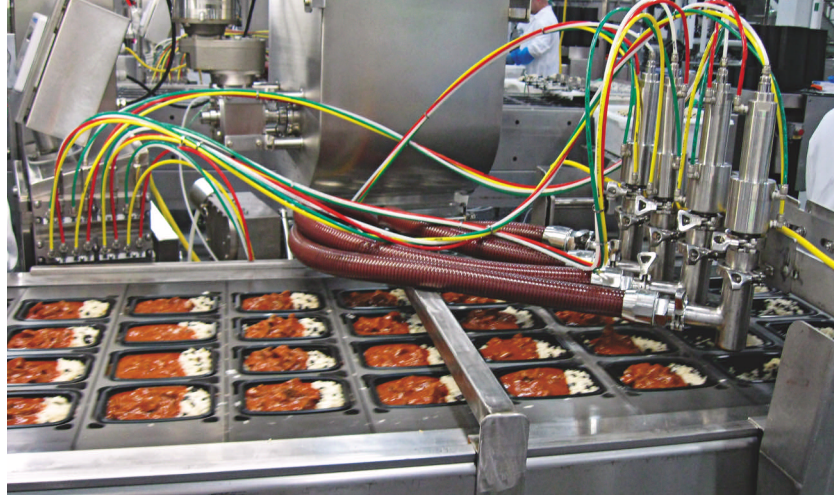
Four piston fillers dispense product as trays travel through the tray sealer.
