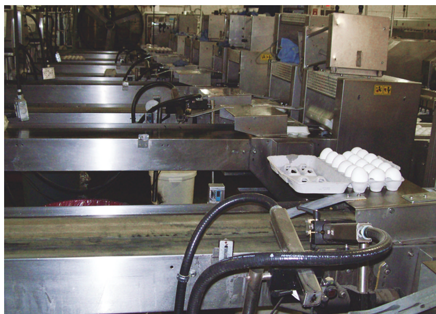
JS West installed new ink-jet printers on all 10 of its egg-packing lines, left. It prints date, lot number and plant number on the edge of each egg carton, above. It packs eggs in both foam and pulp cartons, and had problems with both of them with the old printers. Foam cartons didn’t absorb the ink so the ink wouldn’t dry and would smear, while the pulp cartons would absorb the ink, but the printing was fuzzy.
